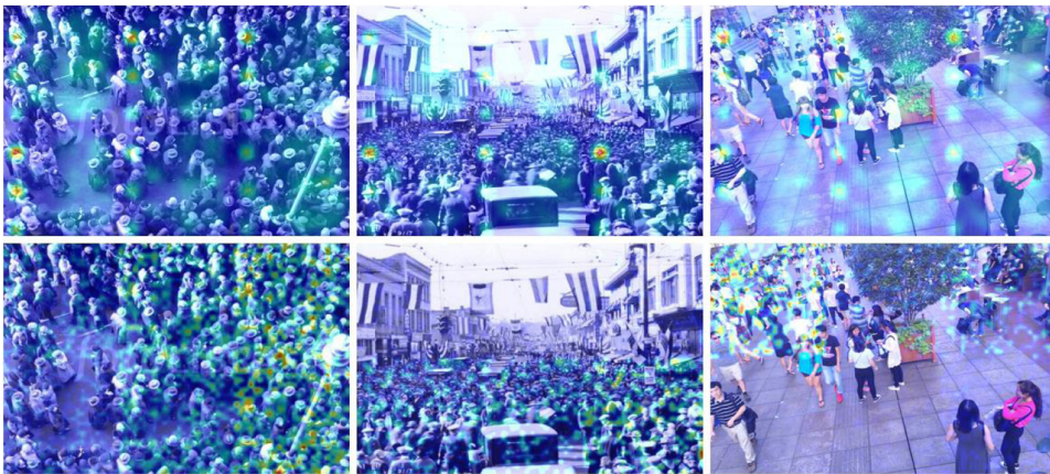
Fig. 8. Comparison of heatmap visualization results generated by the attention module CBAM (the top row) and the HA module (the following row).
